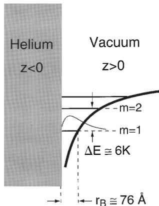
**Fig. 1.** The geometry for an electron trapped at the helium vacuum interface. The Rydberg energy levels along with a typical  $m = 1$  wave function are displayed in the image potential  $V(z) = -\Lambda e^2/z$  for  $z > 0$ .
