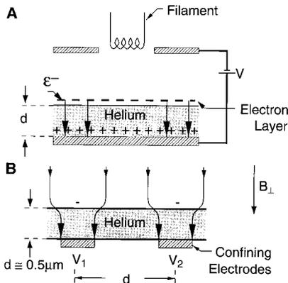
**Fig. 2.** (A) The parallel plate capacitor arrangement for confining a uniform layer of electrons. The holding field  $\mathcal{E}_-$  and the filament for charging are shown. (B) The geometry for a pair of electrons on a patterned substrate. The rough dimensions, the shape of the field lines, and the control gate are included.
